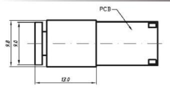
Package for 635nm, 650nm, 780nm, 850nm 5mW laser modules Spot Beam
